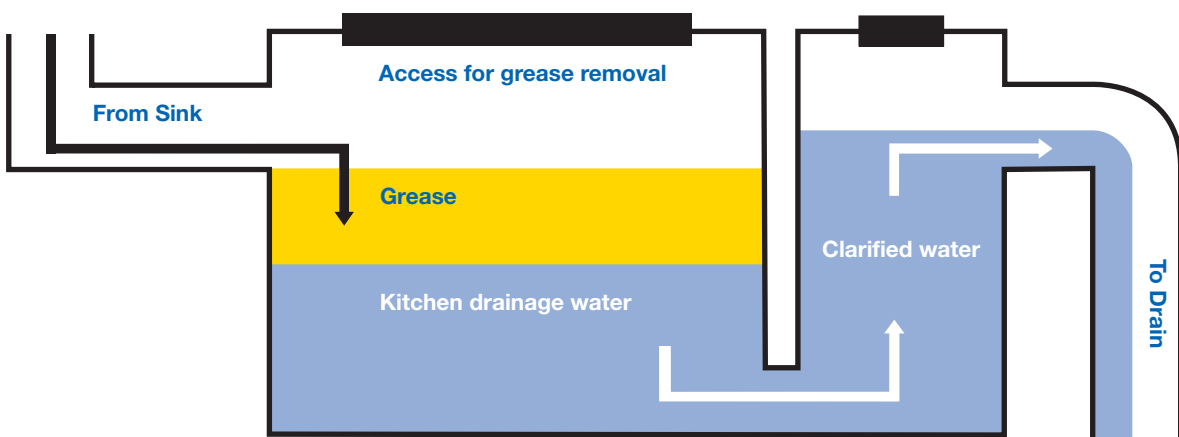
Diagram of an “under-the-sink” grease trap
